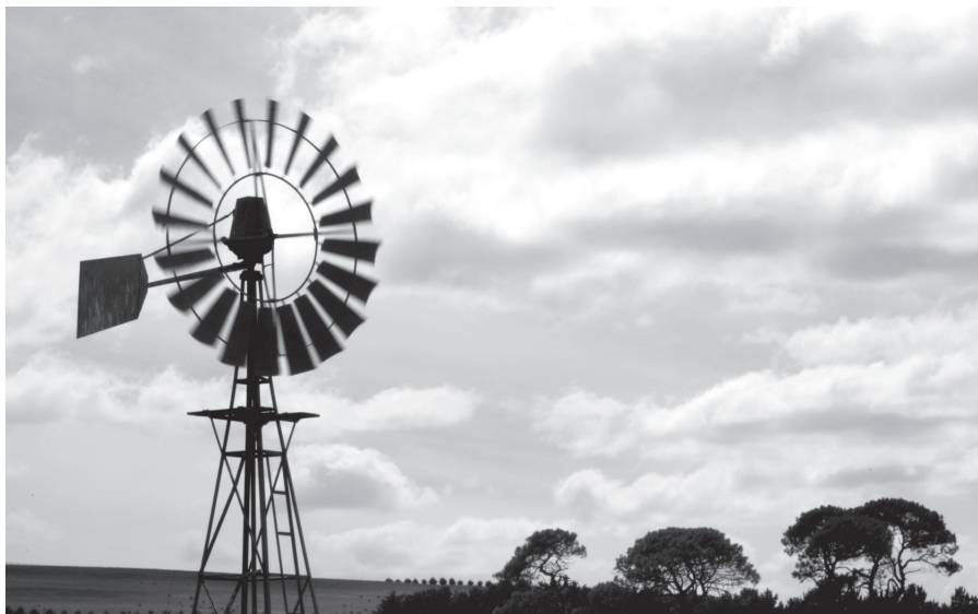
Windmill used for the extraction of groundwater
