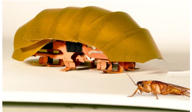
▲ The compressible robot, CRAM with a complaint, yet tough cockroach. †[Source: ©Tom Libby, Kaushik Jayaram and Pauline Jennings. Courtesy of PolyPEDAL Lab UC Berkeley.]
